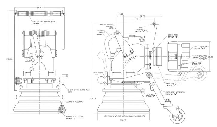
Various options are available on the Model 64810 coupler. The part number system is described to the right. The complete part number is comprised of four parts, as explained in the tables below.
